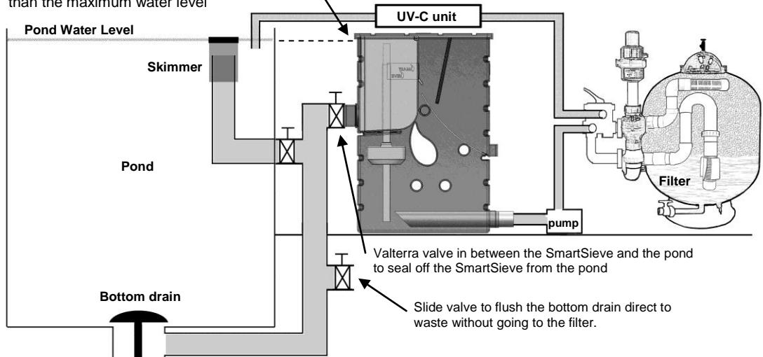
Make sure the SmartSieve is on an equal, level, underground. **The upper edge of the SmartSieve must be 1 cm above the maximum water level.**
