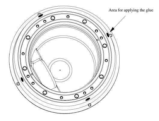
In order to secure the position of the gasket during applying the foil, the seal should be fixed to the body on approx. 4 glue areas (see drawing).
